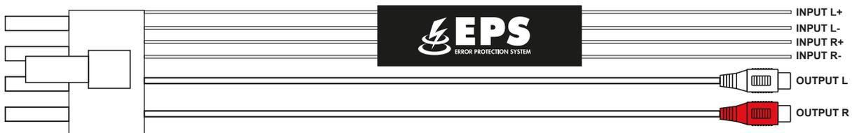
The **OUTPUT** RCA jacks of both wire harnesses provide a linear full-range audio signal for driving additional amplifiers.
