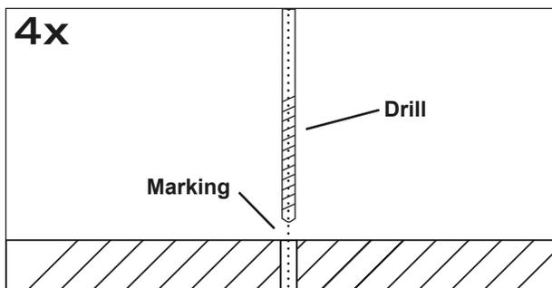
Lay the amplifier aside and then drill the holes for the mounting screws at the marked locations.
