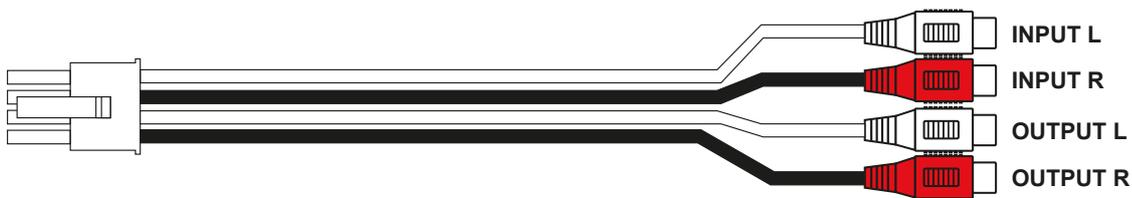
If your head unit does not have RCA preamp outputs, you can use the amplifier's high level inputs as signal input. Simply connect the loudspeaker cables of the head unit to the enclosed wire harness as follows:
