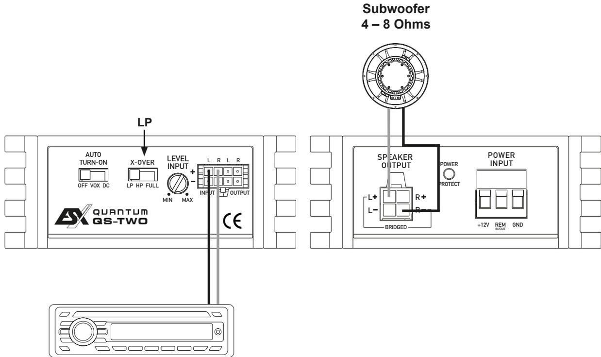
Connect stereo RCA output (L/R or SUB OUT) of the head unit with INPUT (L/R) of the amplifier
