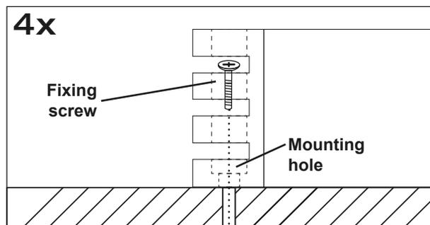
Then uphold the amplifier to the chosen position and fix the screws through the mounting holes into the drilled screw holes.
